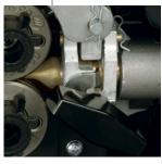
**Gun locking tab** works with guns having corresponding locking grooves to prevent gun from being pulled out if the feeder is dragged by the gun.
