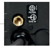
Gas inlet recessed into back of case is protected from incidental contact by the weld cable, ensuring consistent and contaminant-free shielding gas delivery to the gun. **Double-filtered gas valve** helps keep dirt from clogging and affecting gas flow.
